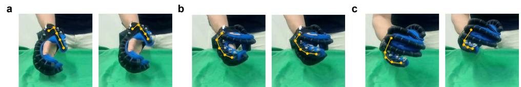
Figure 4. Qualitative results of predictions. Our model accurately estimated finger poses at different angles. (a) Thumb motions. (b) Middle finger motions. (c) Pinky finger motions.
