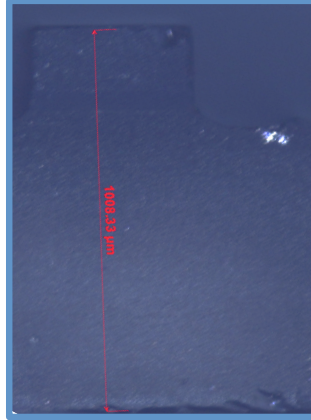
FIGURE 4.6: (a) Concave feature properties, dimensions are in microns. (b) Optical microscope images of the finished plinth after coating. (c) Optical microscope image of the plinth, side-on. The plinth extends 250\mu\text{m} above the rest of the substrate (c) A 4\times 4 grid, each of side 50\mu\text{m} , is FIB milled onto the planar mirror after coating. An orientation mark and guides are also milled, to locate this region of interest
