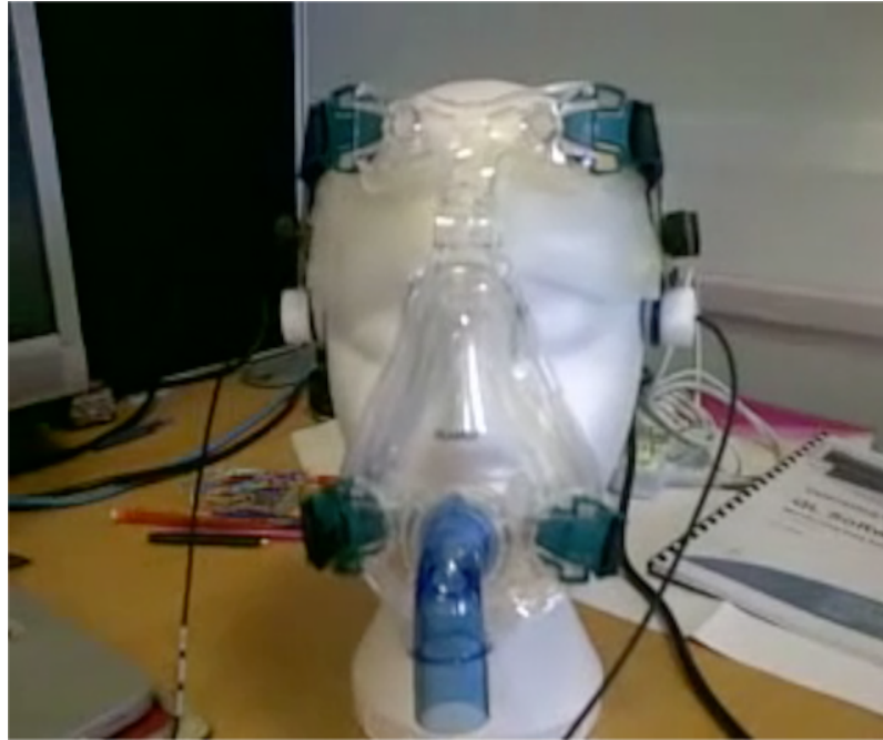
Figure 6.2 Face mask was selected for its tight seal, easy quick release and its comfort.
