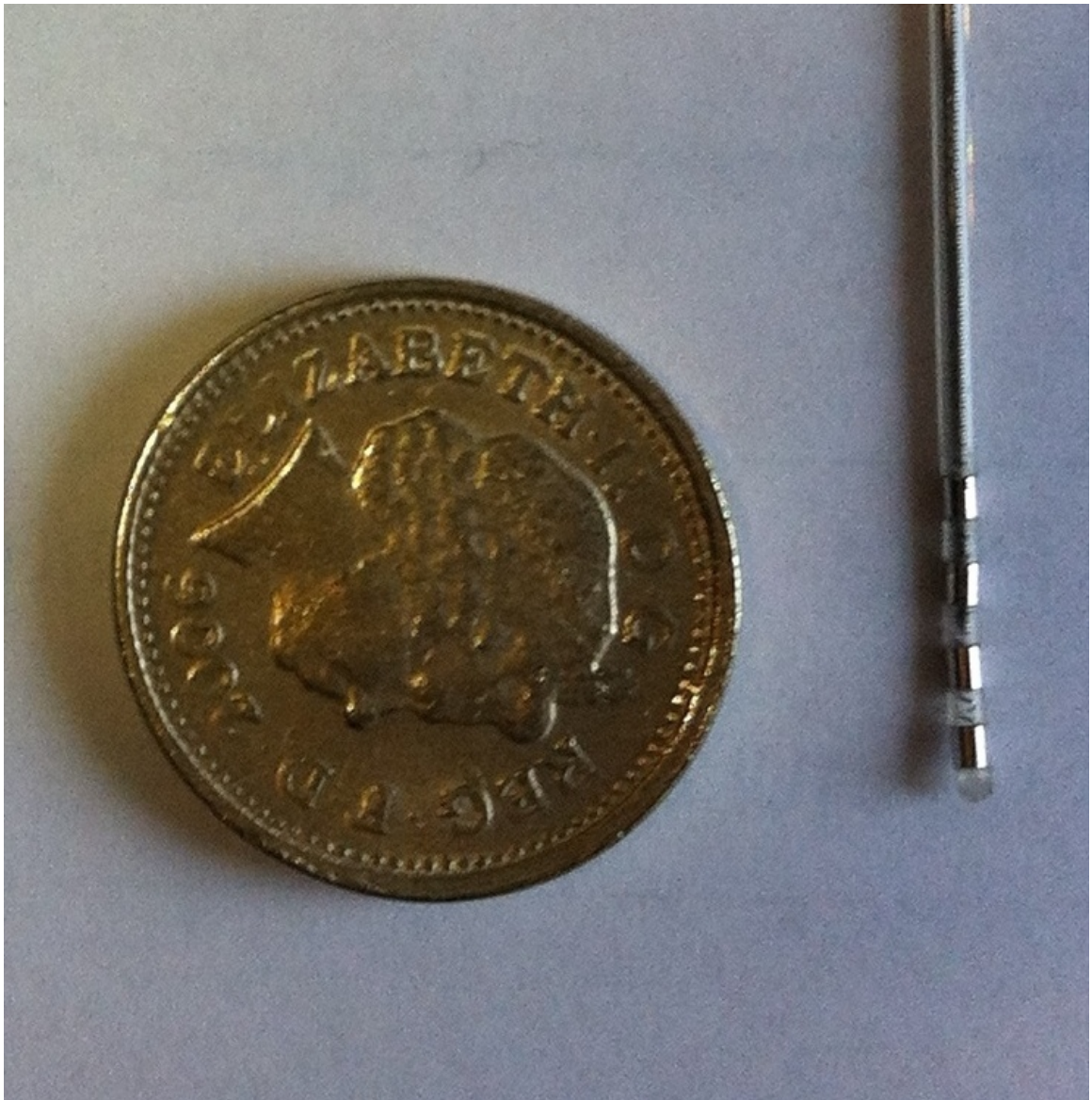
Figure 6.10 Physical comparison of Medtronic Model 3387 deep brain stimulation electrode to 1 pound coin.
