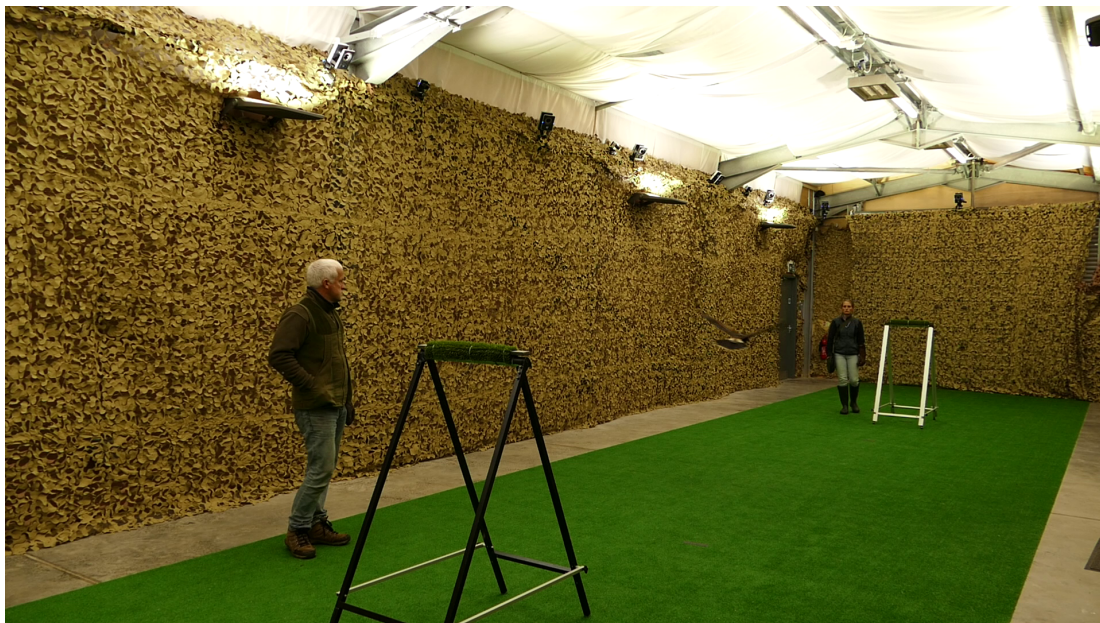
Figure 3.4: Flight lab experimental setup. Two A-frames were positioned 12m (shown), 9m, 7m, and 5m apart as experimental conditions. Twenty motion capture cameras positioned around the perimeter room around 3.5m high, and LED lights and white fabric on the ceiling mimic overcast daylight conditions.
