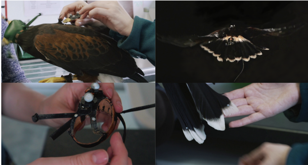
Figure 3.2: Photograph of markers and equipment. Clockwise from the top: the backpack marker plate being attached to a hooded Harris hawk prior to the experiment; the backpack and tail mount marker sets during an example flight (photograph courtesy of AngleSharp Media); the modified hood with markers; 3mm markers attached to the tail feathers.
