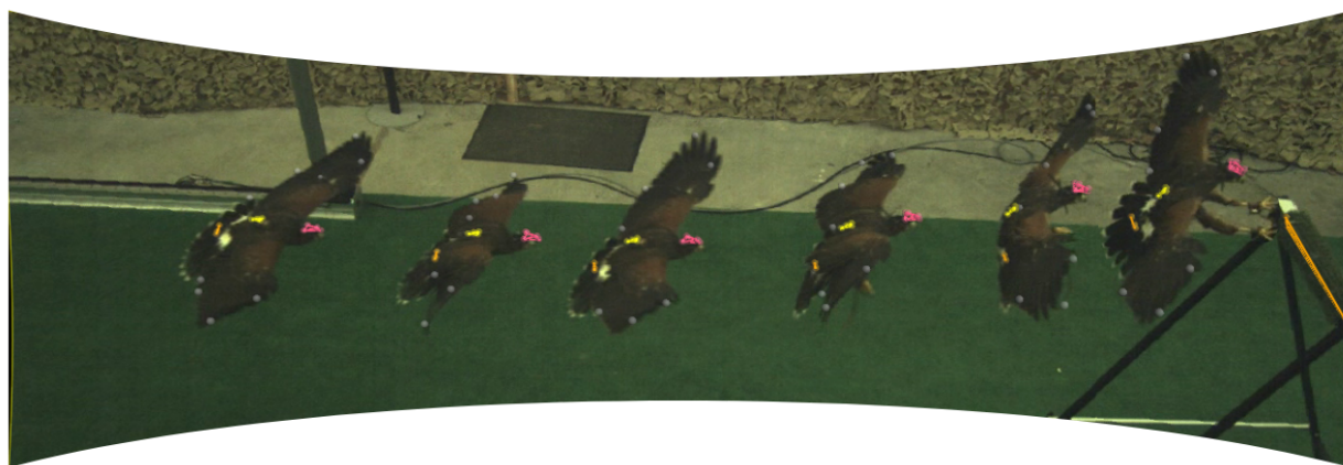
Figure 3.5: Marker set from motion capture overlaid onto reference footage. Markers coloured by type: hood (pink), backpack (yellow), tail mount (orange), feathers (grey) during the glide and rapid pitch-up. The stationary markers on the perch are linked with an orange bar.
