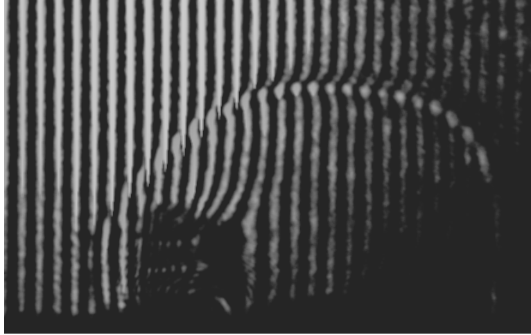
Figure 8.1: Zoomed-in interferogram taken 32.5 ns after drive beam. Significant bending of fringes is seen near the target; this is due to the high density of the shock at early times. Most of the fringes in the high contrast region are not broken and can therefore be processed using the standard Fourier transform method as shown in the top left of Figure 8.2
