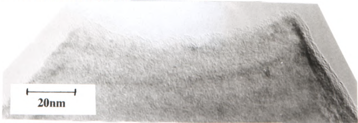
c) Emitter which has been oxidised 7 times - Wedge-like apex Tip radius is ~5nm
