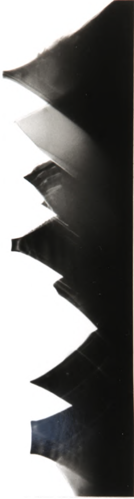
Figure 5.12 - TEM micrographs comparing tip-to-tip uniformity for an under-etched FEA and an FEA etched until the oxide masks have started to fall off
