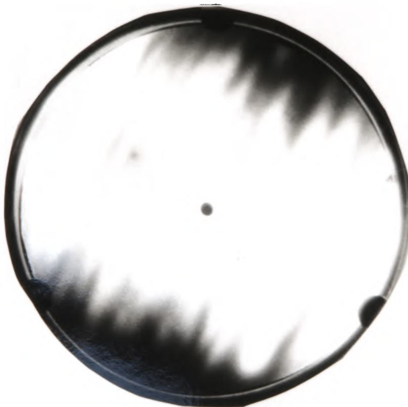
c) FEM image from same tip at 1500V This image was taken before a field emission run was carried out. Emission appears to be localised along blade.
