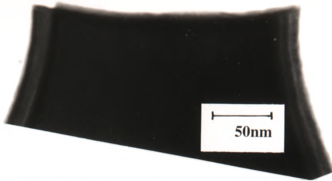
a) Tip 1 - Wide flat-topped emitter observed at centre of sample, where etch rate was the slowest (Top is \sim 0.2\mu\text{m} wide)
