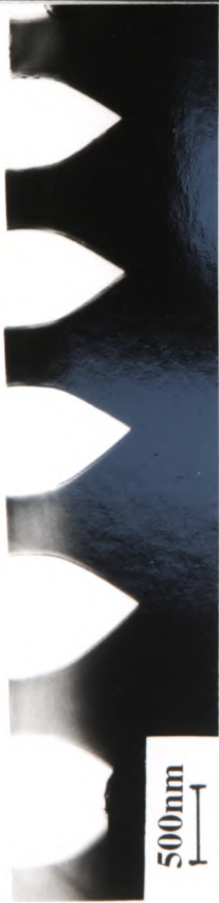
a) Low-magnification image of several flat-topped emitters All tips have the same basic height and geometry.
