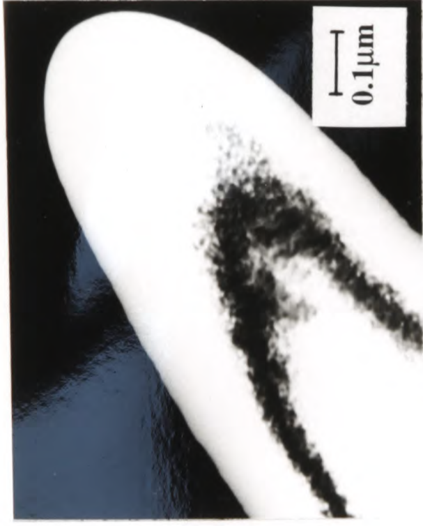
b) Dark Field image of same tip Note tip end is smooth and round
