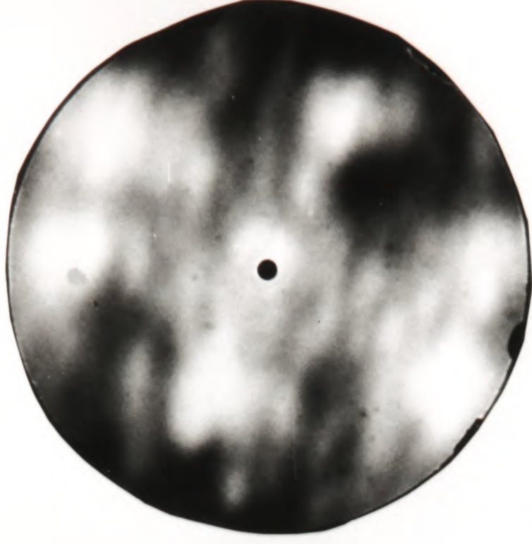
c) FEM image at 1090V Note that some spots are much larger and brighter than other spots. Image is less uniform than for FEM image obtained from uniform tip shown in Figure 8.6c.
