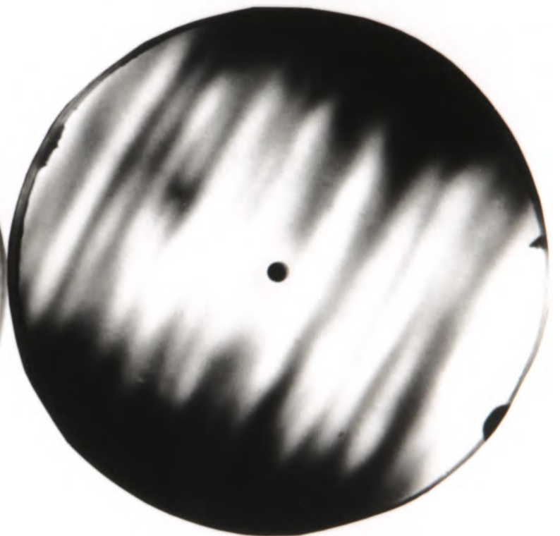
d) FEM image from same tip at 1508V This image was taken after a field emission run was carried out to \sim 1\mu\text{A} . Note that FEM image is less bright following emission.
