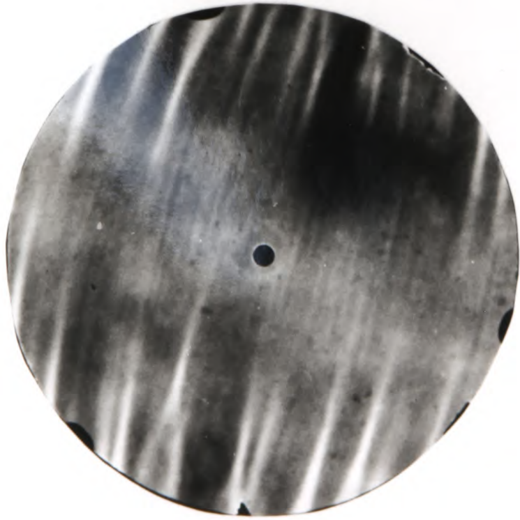
a) FIM image at 7.7kV Note streaks across image indicating that tip is blade-shaped.
