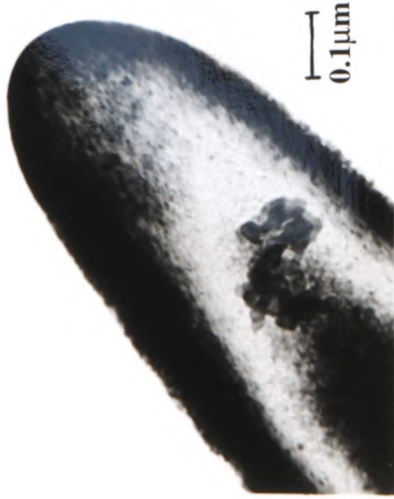
a) Bright-Field image of tip Tip radius is \sim 100\text{nm} Note tip end is smooth and round
