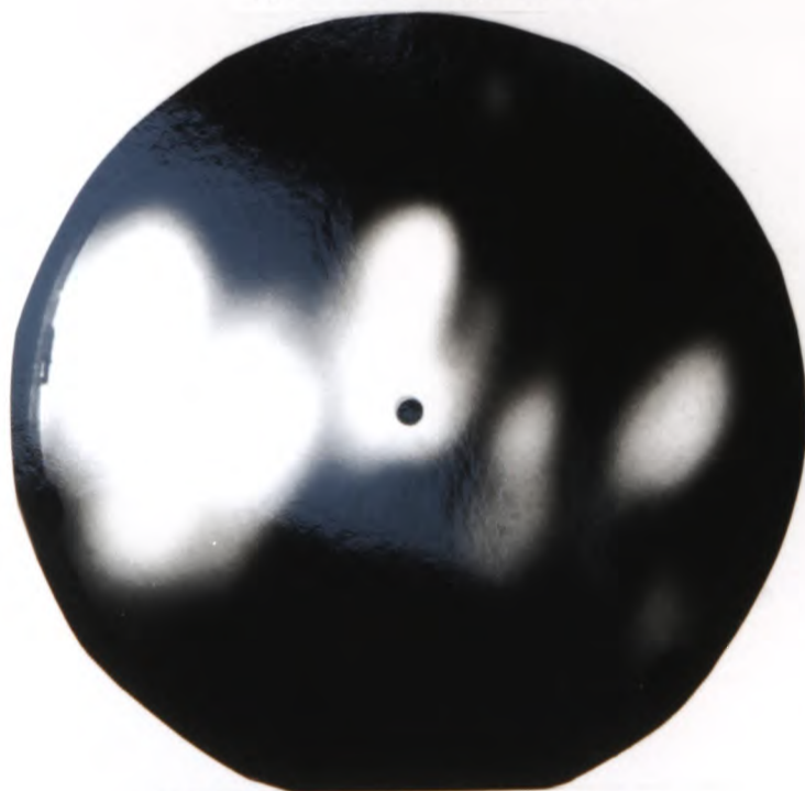
e) FEM image at 748V Following emission run to \sim 0.1\mu\text{A}
