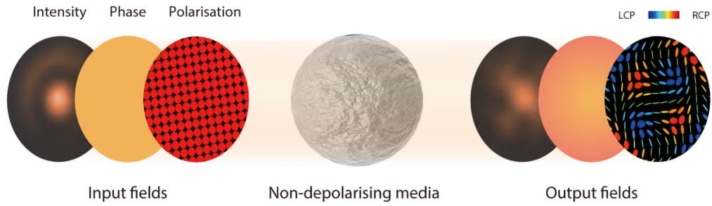
Figure 5.1: Non-depolarising media. Illustrations of how non-depolarising media affect the spatial distributions of intensity, phase and polarisation fields. Retardance in non-depolarising media affects phase and polarisation, while diattenuation impacts phase, polarisation, and intensity 12,121–123 . The spatially varying distributions of intensity, phase, and polarisation fields before and after passing through the non-depolarising media are shown. Circular planes represent the beam's spatial profiles in each of the three domains.
