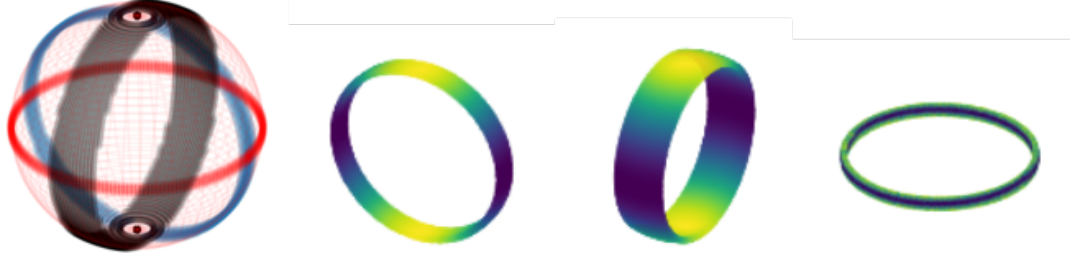
Figure A.10: Parts of a Newton sphere with a \cos^2 \theta distribution used to be fitted by the least squares fitting programme. Each portion of the Newton sphere reproduces the data well.
