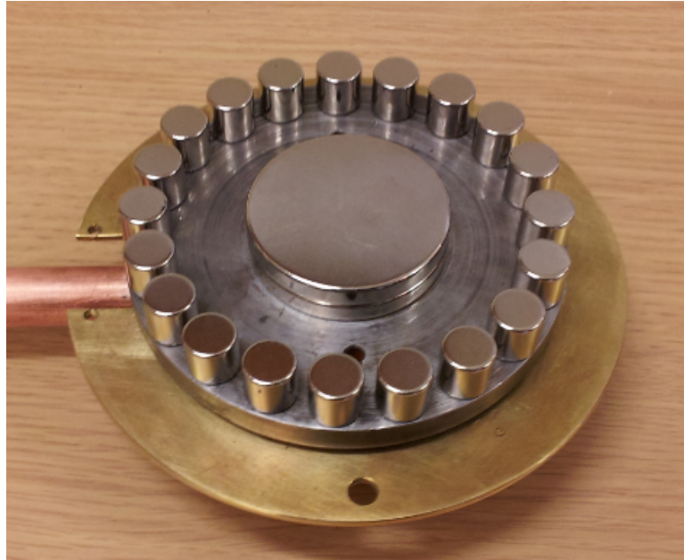
Figure 4.4: The inside of the ZnO magnetron and the spatial arrangement of the NdFeB magnets.
