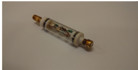
Langmuir probe in a ZnO magnetron plasma
