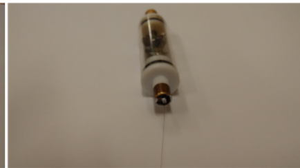
Langmuir probe in a ZnO magnetron plasma
