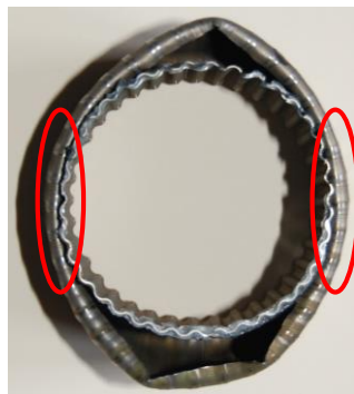
Figure 4.30. Self-contact of Cor2.
