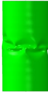
(a) Buckling analysis when displacement was 2.5 mm
