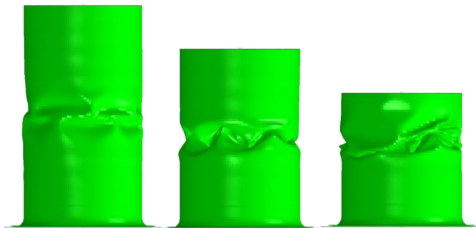
(b) Numerical deformation with displacements of 10 mm, 30 mm, and 50 mm respectively.
