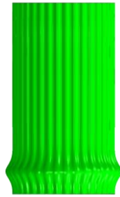
(a) Buckling analysis when displacement was 2.5mm
