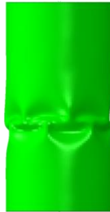
(a) Buckling analysis when displacement was 2.5 mm
