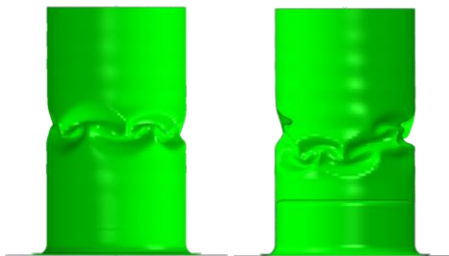
(c) Side and cut view of inverting analysis when displacement was 16 mm
