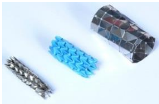
Figure 2.11. A novel origami folding aortic stent graft.
