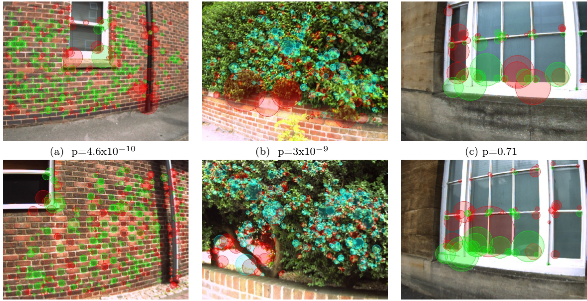
Figure 4.6: Some examples of remarkably similar-looking images from different parts of the workspace that were correctly assigned low probability of having come from the same place. Results were generated using the accelerated likelihood calculation. The examples represent typical system performance. This result is possible because most of the probability mass is captured by locations in the sampling set – effectively the system has learned that images like these are common in the environment. Words present in both images are shown in green, others in red. (Common words shown in blue in (b) for better contrast). The probability that the two images come from the same place is indicated between the pairs.
