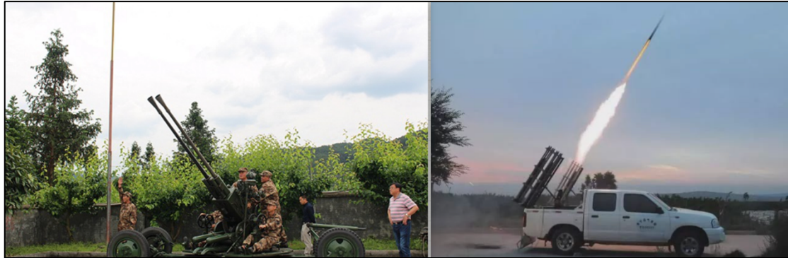
Figure 26 Cloud seeding operated with former military devices such as the cannon and rocket launchers.
