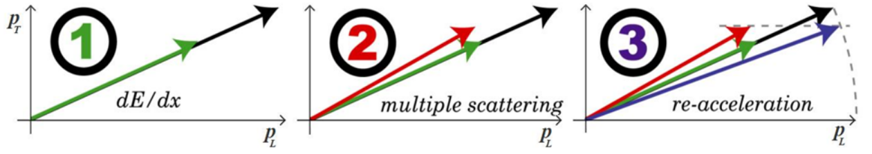
Figure 1.2: The technique of ionization cooling whereby a beam of muons is directed through an absorber followed immediately by a radio-frequency (RF) accelerating cavity.
