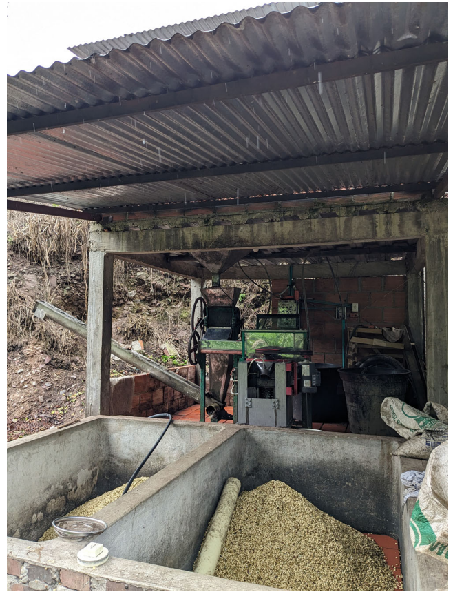
FIGURE 2 A roofed beneficiadero , where harvested coffee cherries are brought for processing, at the Bellavista farm, in a vereda (rural district) of the municipality of Arboledas, Norte de Santander. In the foreground are two cement fosas (basins); in the background, a coffee-pulping machine. (Javier Lezaun and Lina Pinto-García) [This figure appears in color in the online issue]
