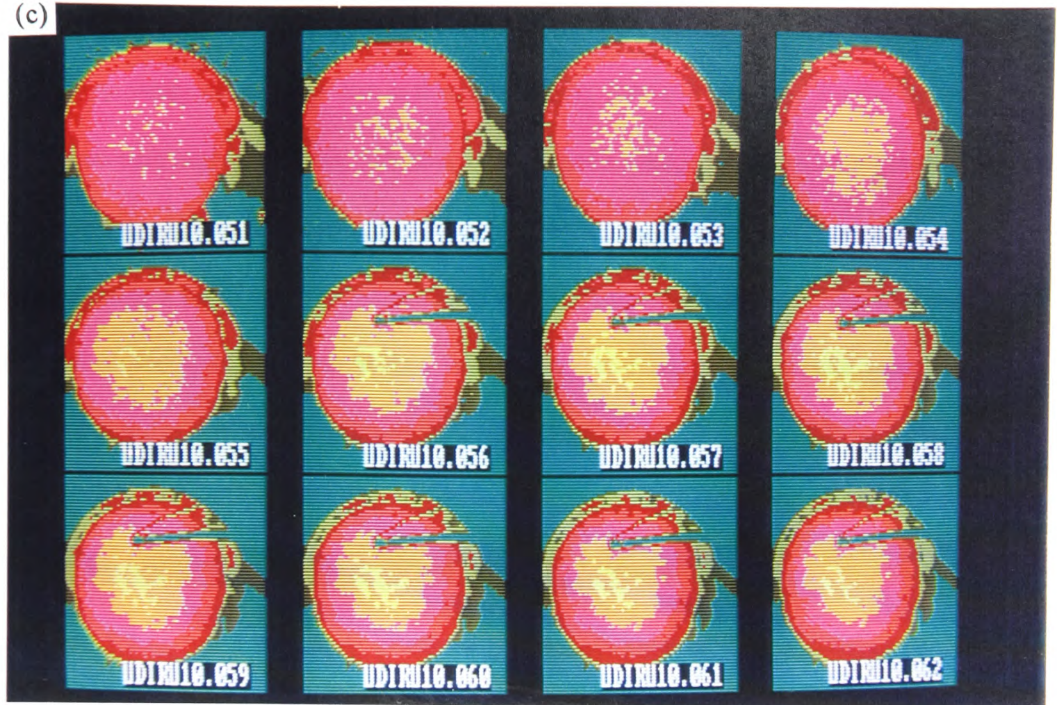
cont... Fig 5.7 Sequence of thermal images taken from run 10 assuming \epsilon_0=0.3 ; (a) at the beginning of the run; (b) in the middle of the run; and (c) just after the end of the run respectively.
