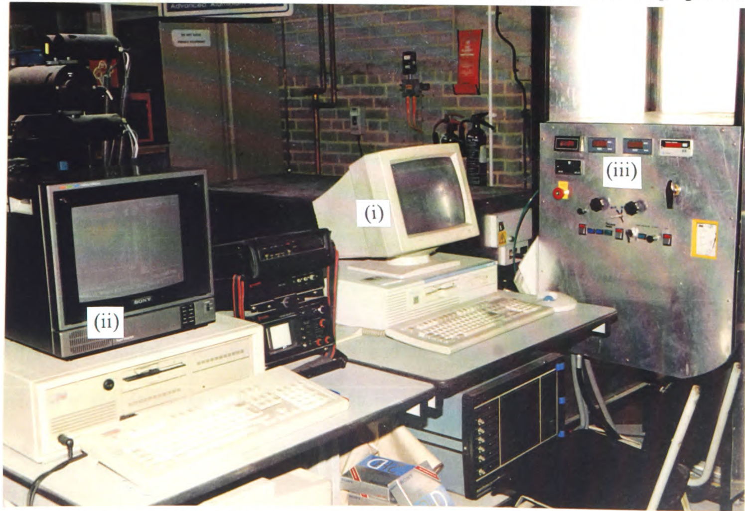
Fig 3.6(b) Photograph of the spray forming control equipment showing; (i) computer to control the thermal imaging camera, (ii) computer to control the datalogger and (iii) instrument panel to control overpressure, gas flow rate, stopper rod and cyclone.
