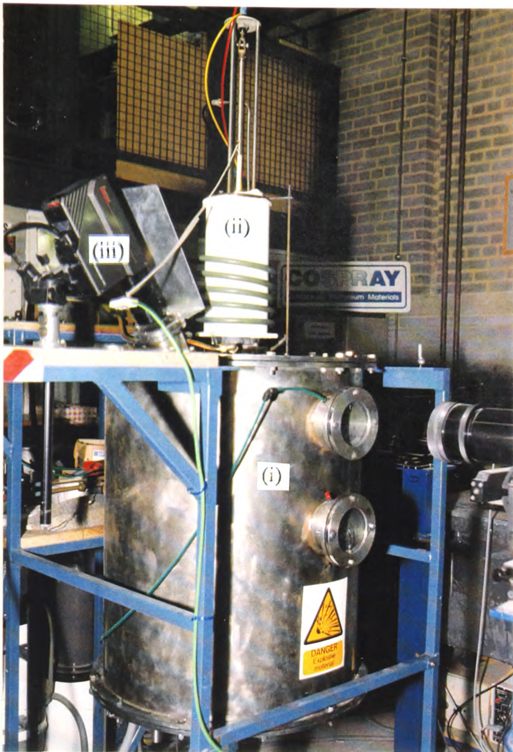
Fig 3.6(a) Photograph of the spray forming arrangement showing; (i) the spray forming chamber, (ii) the melting arrangement and induction coil and (iii) thermal imaging camera.
