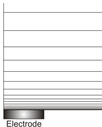
Figure 3.3 – Mesh Spacing representation in the Z direction.
