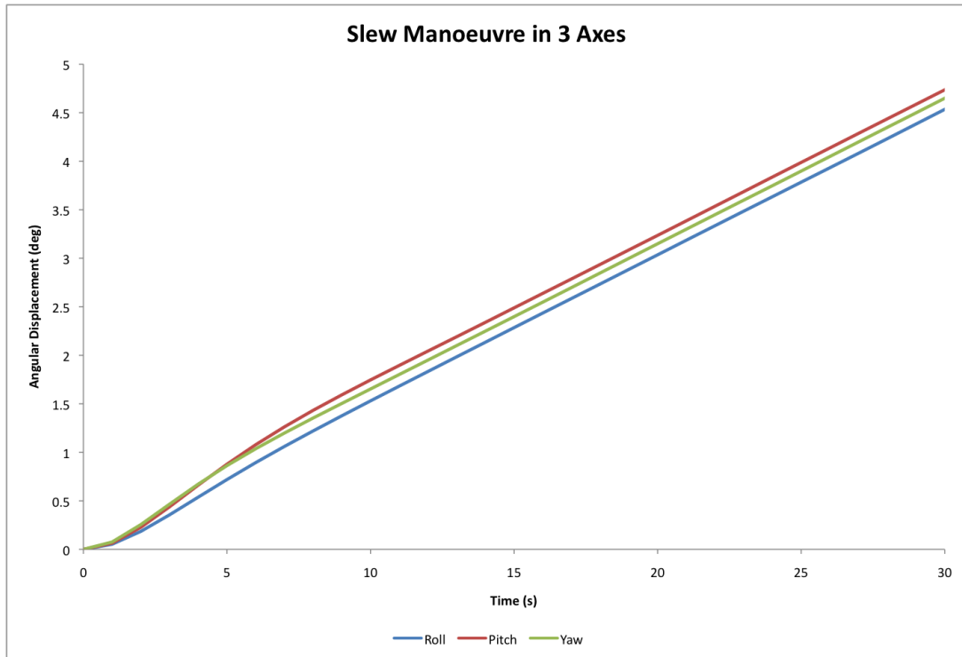
Figure 6.12: Slew manoeuvre in all 3 axes using model predictive control
