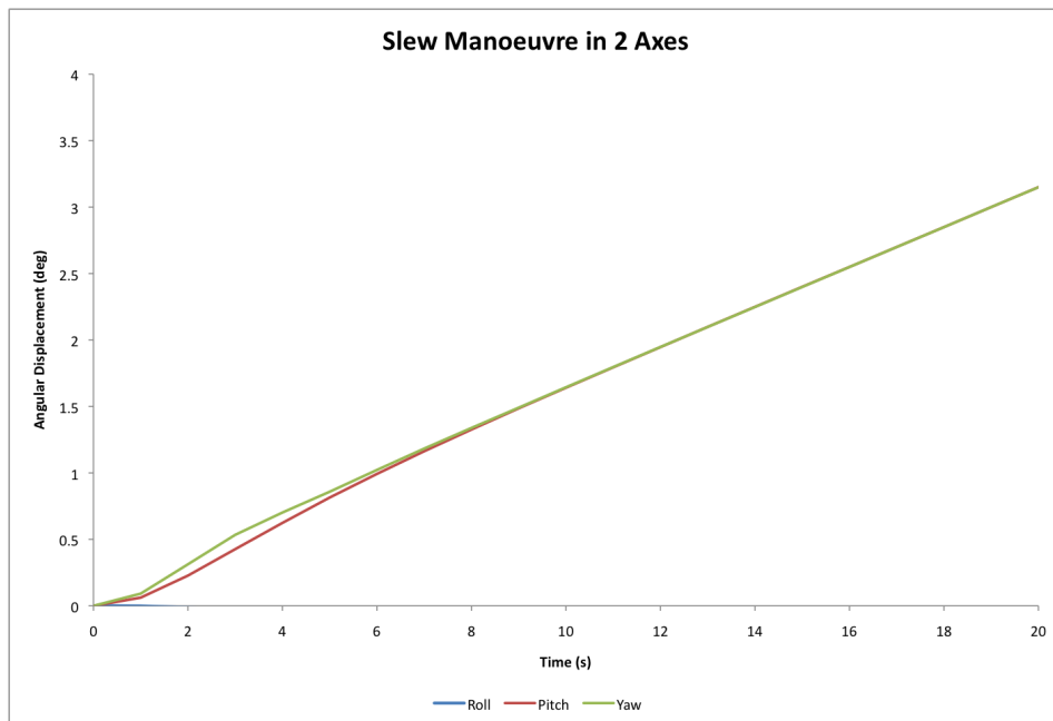
Figure 7.8: Slew manoeuvre in pitch and yaw axes using PD control
