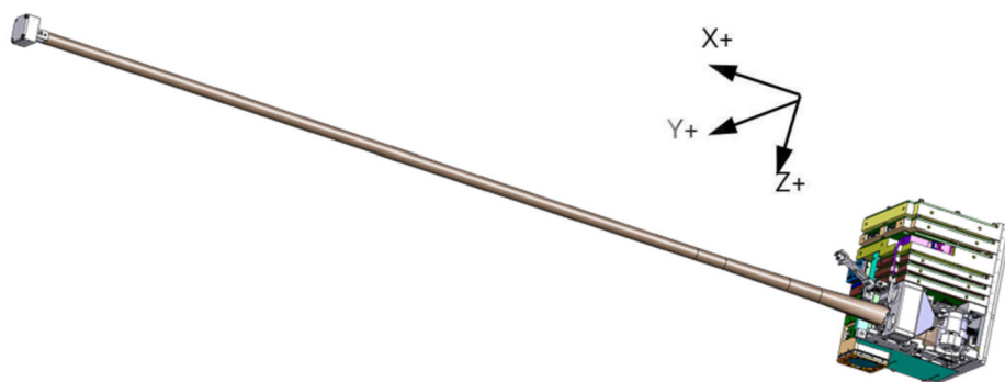
Fig. 4 Illustration of the RadMag payload with magnetometer boom deployed. The MAGIC outboard sensor is visible at the end of the boom. The platform coordinate system is also shown, with the x-direction aligned to the boom. The boom deploys perpendicular to the plane containing the solar panels in the anti-sunward direction
