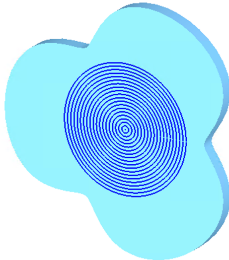
Figure A.2: 30 discrete cylindrical surfaces composed of 720 azimuthal points at 10 regularly spaced longitudinal intervals are created with radii between 0.1 mm and 47.5 mm, as per Point 2.
