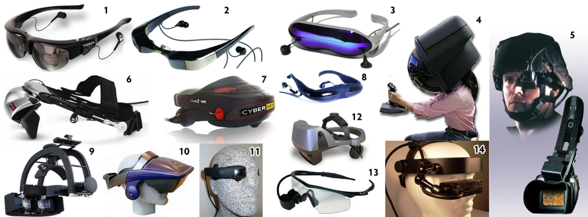
Figure 1.4: A selection of head mounted displays (HMDs) currently available, ranging from simple video displays to 'see-through' displays in monocular and binocular varieties. In numbered order they are from the following manufacturers [152, 103, 141, 149, 123, 37, 23, 60, 130, 126, 150, 108, 21, 82].
