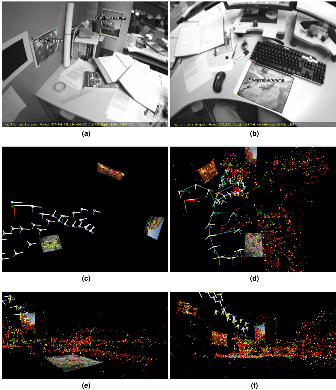
Figure 6.14: (a,b) Images from the cluttered desk sequence. (c) An overhead view of the map. (d) Another overhead view showing the bidirectional tree structure and the map points along with the detected objects. (e,f) Close-up views of the Grasshopper poster, showing that it is well localized with the surrounding map points (see video exp4_cluttered_desk.avi ).
