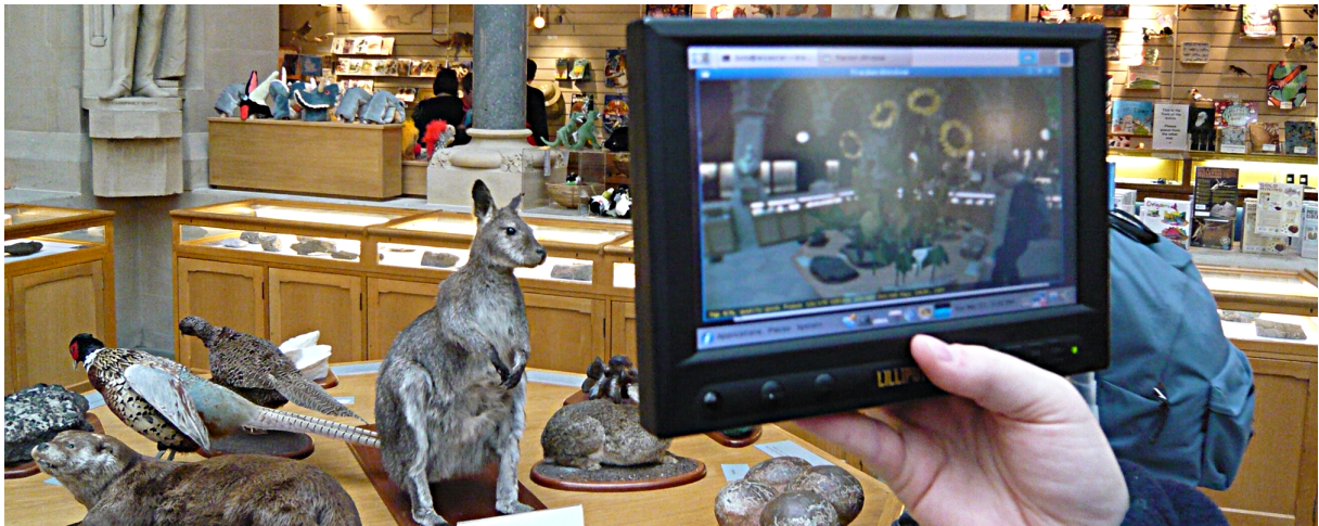
Figure 2.2: An example of a magic lens. The AR model of a bunch of sunflowers can be seen placed on the table in the display.
