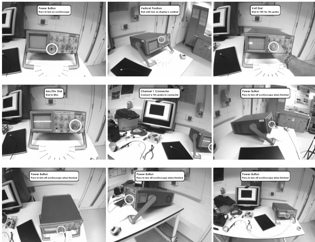
Figure 6.19: In this AR oscilloscope tutorial, AR elements are placed with respect to locations within the object's extent. As the user advances through the tutorial different overlays are displayed (see video exp7_oscilloscope.avi).
