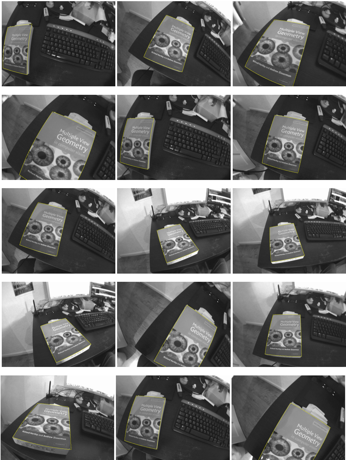
Figure 6.7: Sample of 15 out of the 29 keyframes where the book was detected, with the calculated homography represented by the book's outline.
