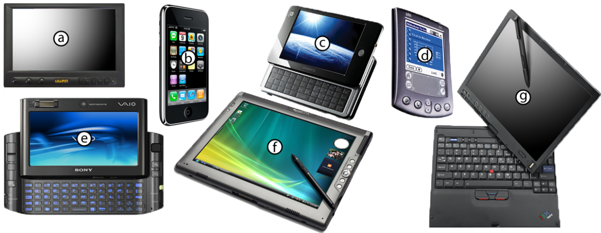
Figure 1.5: A selection of touch screen devices. (a) an 8 inch touchscreen display from Lilliput [80], (b) Mobile phone and media player from Apple [4], (c) a MID from Gigabyte [48], (d) a PDA from Palm [112] (e) a UMPC from Sony [141], (f) a slate PC from Motion Computing [101], and (g) a tablet PC from Lenovo [73].
