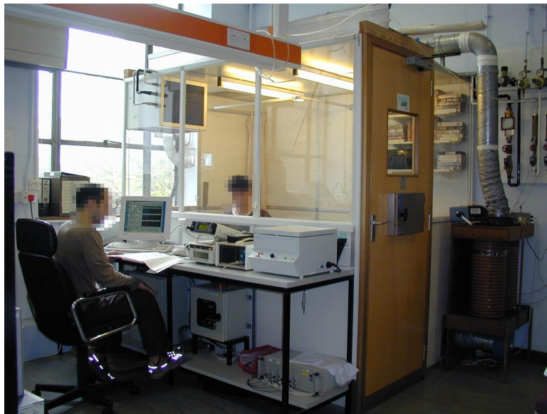
Figure 3.4: The custom-built study chamber in the Department of Physiology, Anatomy and Genetics, prior to the covering of internal surfaces with reflective material.
