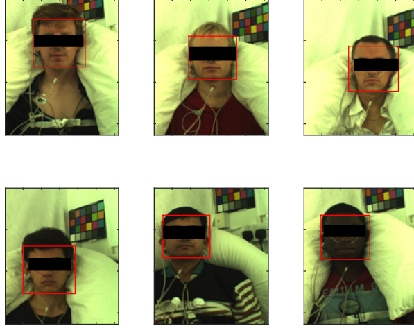
Figure 4.5: Figure showing face detection using the modified Viola-Jones algorithm for the six different skin phenotypes. Detected face bounding box shown in red.
