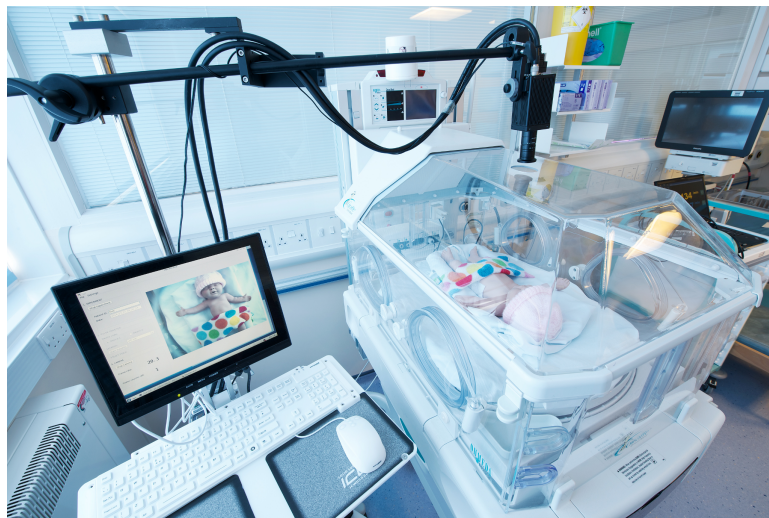
Figure 3.1: Monitoring set-up used in the Neonatal study showing the video camera placed above the modified incubator.
