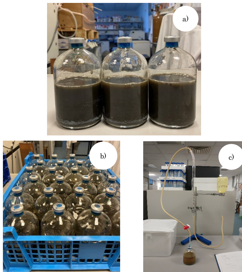
Fig. 3.2 a) BMP apparatus showing a set of 250 ml glass bottles sealed with rubber stoppers and aluminium caps. b) A rack of BMP bottles to be incubated in an orbital shaking incubator. c) A eudiometer for biogas volume measurement.
