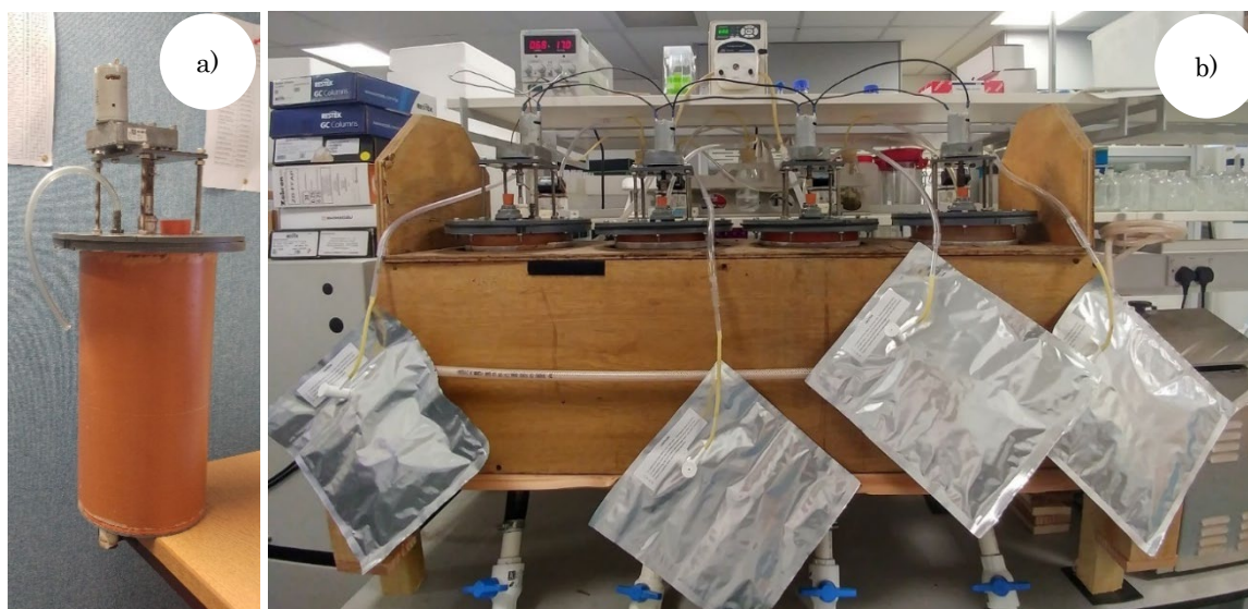
Fig. 3.3 Laboratory-scale CSTR digesters used in the research. a) a 5 L digester. b) A set of four 5 L digesters in a heated water jacket connected to a temperature-controlled water bath.
