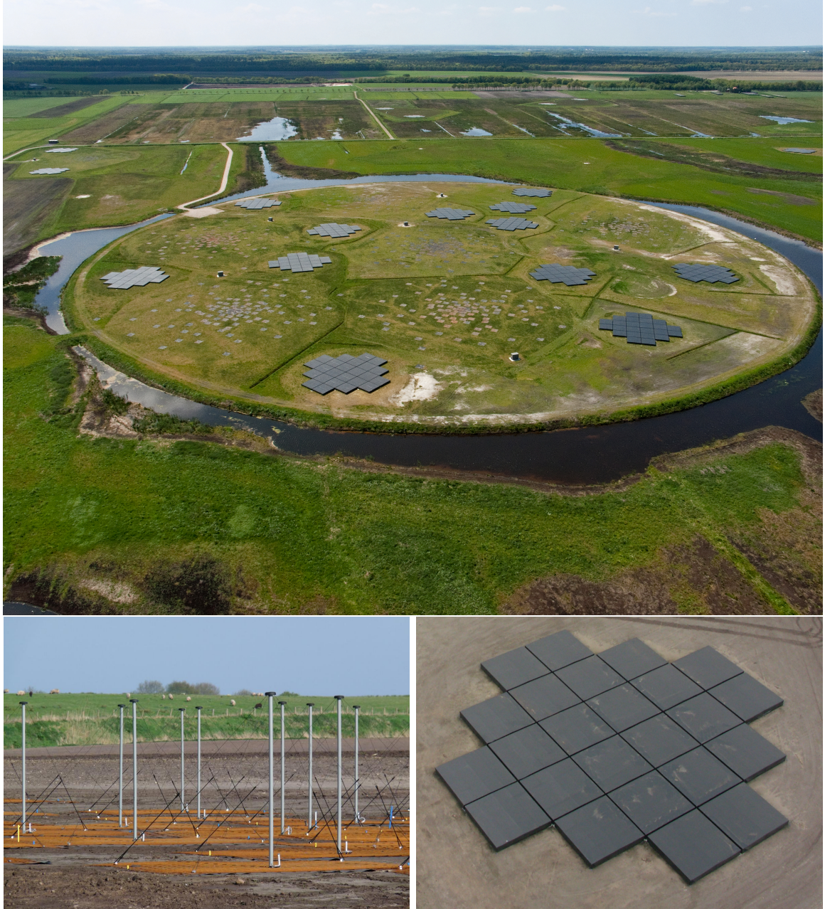
Figure 2.3: Top : an aerial view of the land that houses 6 of the LOFAR stations. Bottom left : the Low-Band Antennas (LBAs) that observe 30-80 MHz. Bottom right : the black casings that cover the High-Band Antennas (HBAs) that observe 120-240 MHz. Image credits : aerial view - Top-Foto, Assen; LBAs and HBAs - ASTRON.
