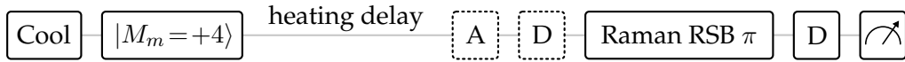
Figure 8.1: Pulse sequence used for measuring the heating rate, applicable to one or two ions. After ground state cooling, we prepare the |M_m = +4\rangle state, and subsequently wait for a varying amount of time to allow for heating. We then apply either a red or a blue Raman sideband pulse, the latter in the form of a red Raman sideband pulse preceded by the microwave transfer \pi -pulses A and D , which eliminates the need to change the Raman laser frequency. Lastly, we apply another D pulse and read out from the stretch qubit, i.e. |M_n = +3\rangle and |M_m = +4\rangle .
