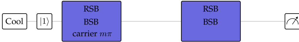
Figure 7.3: Single-ion pulse sequence used for measuring the AC-Zeeman shift generated by the sideband microwaves. We apply the carrier drive in the first half of the gate and scan its frequency to find the shifted qubit transition.
