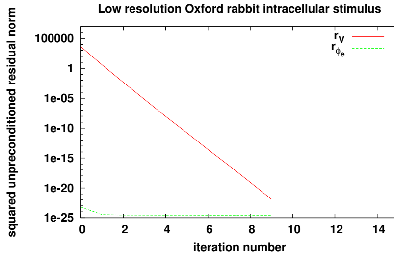
Figure 5.7 Evolution of the residual associated with each of the magnitudes of interest ( V and \phi_e ) at onset of stimulus. Simulation described in Table 5.2-A with low resolution mesh without bath and PE-ILU solver.
