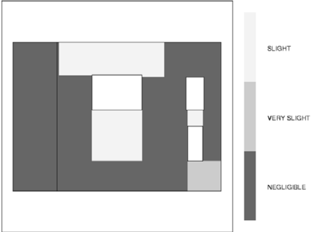
Figure 5-12: Damage to east façade predicted by combined analysis (Analysis 2)
