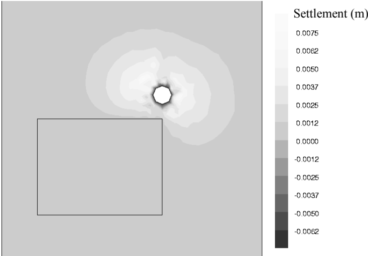
Figure 5-28: Surface settlements for combined model with elastic raft
