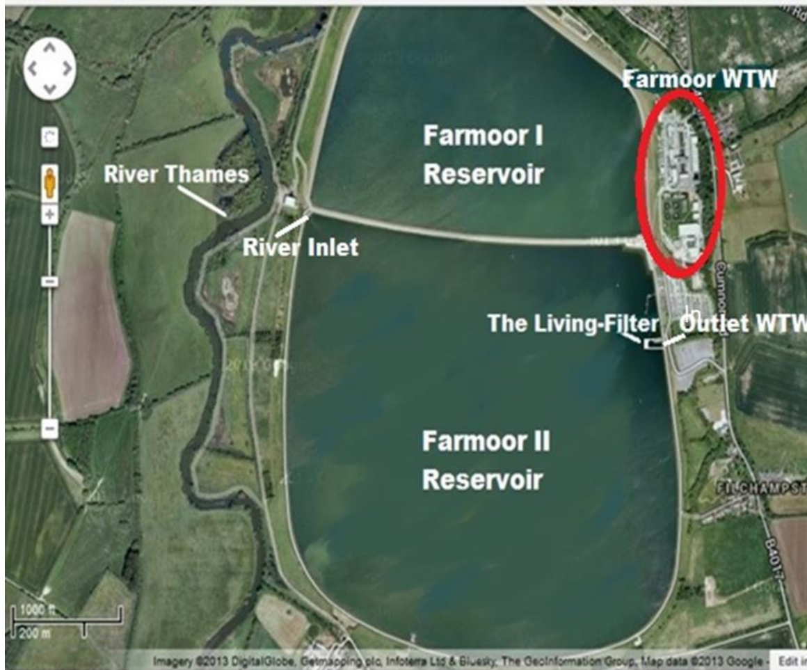
Figure 1.1 Aerial image of Farmoor reservoir (I and II), showing the location of the River Thames intake, Living-Filter and outlet (or intake) to the WTWs. Farmoor II reservoir and Living-Filter morphometric data (Google Maps, 2013).
