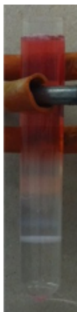
Figure E1- A CsCl column of adenovirus separated from lysed cells after centrifugation at 25,000 rpm for 1 hour 30 minutes.
