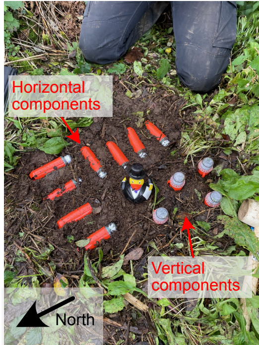
Figure S1 – Example field deployment of 3-component site. Note that this example is for a “stacked” site, where four sensors were deployed in combination for each channel. Typically, most sites only comprise of either one or three nodes (for a Z-only or ZNE sites, respectively). Rubber duck and a person’s knees are included for scale.
