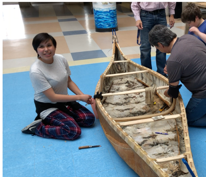
Fig. 5. Trinity lashing thwarts to the gunwales
