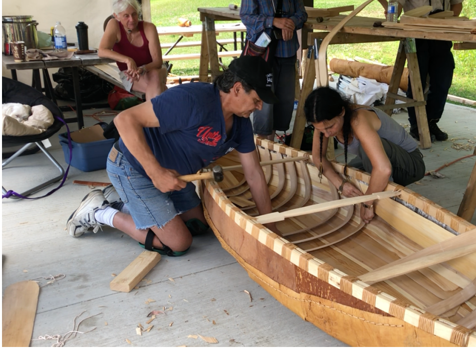
Fig. 8. Chuck and Kathy installing ribs
