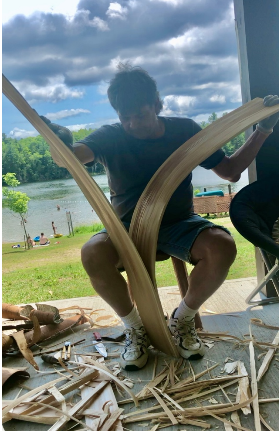
Fig. 6. Chuck splitting cedar sheathing
