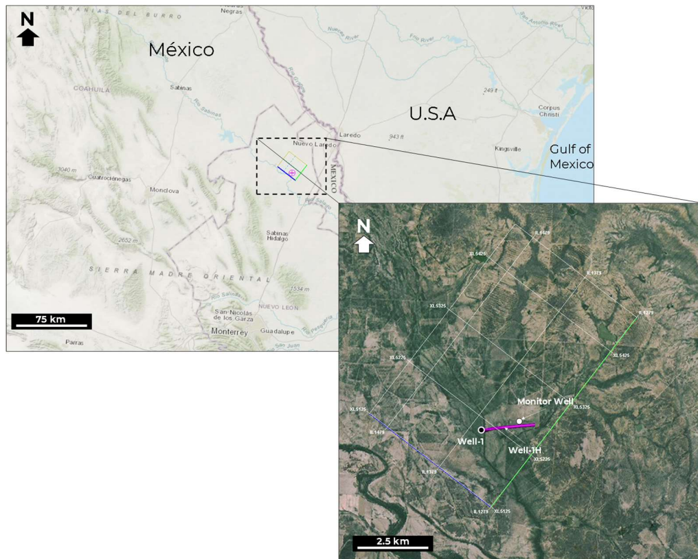
Figure 5.12 Location at Well-1, Well-1H, and monitor well for microseismic survey
