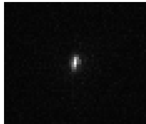
Figure 6.7: Single ion of calcium in Liverpool trap.
