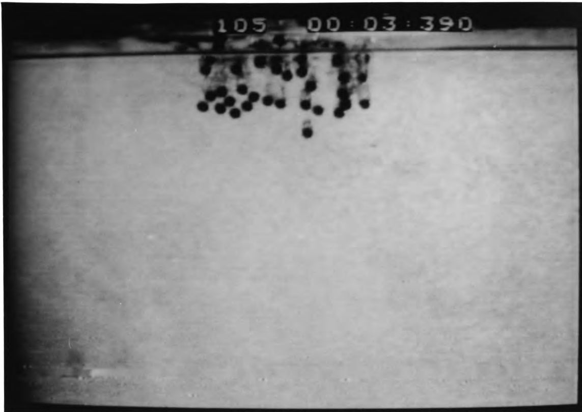
Figure 5.2: A Close up of a Normal Plume 0.02s after entering the Water Pool taken from Experiment a5.
