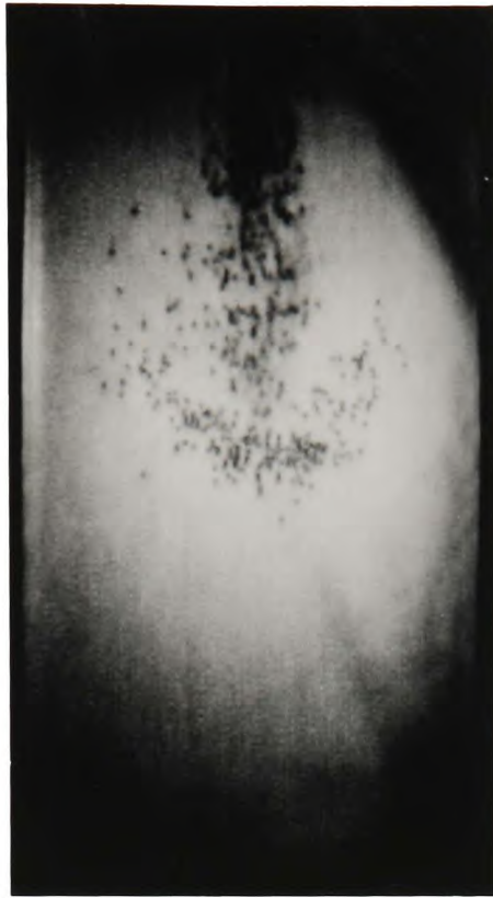
Figure 5.10: A Normal Plume 0.45s after entering the Water Pool taken from Experiment a2.
