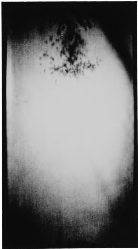
Figure 5.9: A Normal Plume 0.25s after entering the Water Pool taken from Experiment a2.
