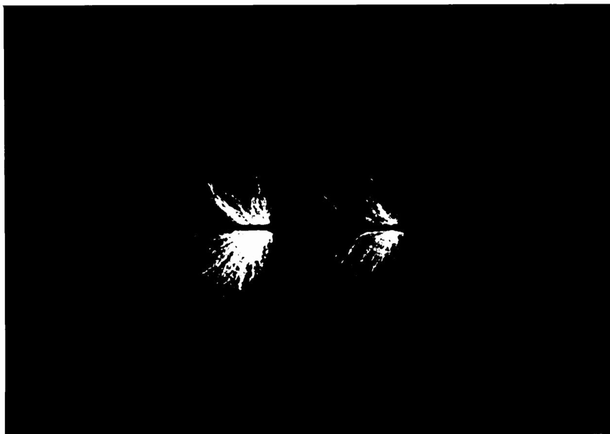
Fig. 6.33 Light stripes observed for a pull-out test on a pair of transverse members spaced 50 mm apart (test no. 43), after 6.02 mm displacement between the pull-out box and deflector bar
