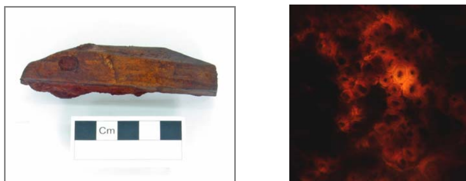
Figure 19: Find no. 32 before conservation. Photomicrograph of ring porous cell arrangement showing intact early wood cells (TS x40). Cell lumen filled with iron corrosion products.
