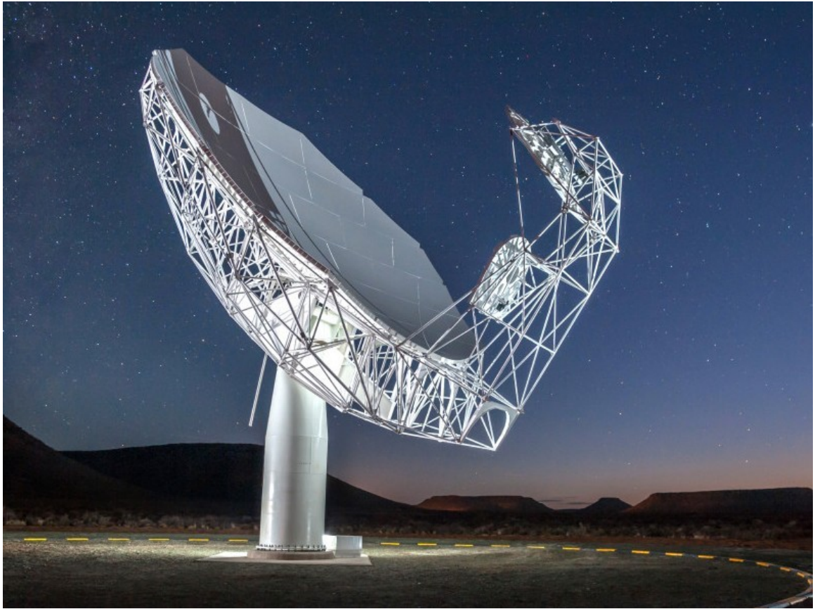
Figure 2.1: This MeerKAT antenna is an example of a parabolic dish which will be used in the mid-frequency array. Credit: Photowise
