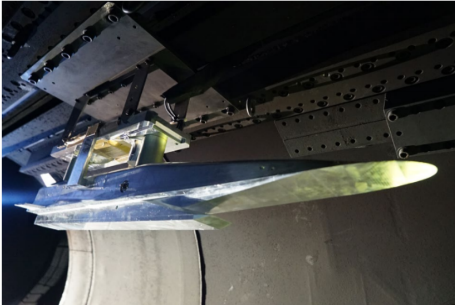
Fig. 2.14 MoDKI model suspended on electromagnets in JAXA HIEST [98]
