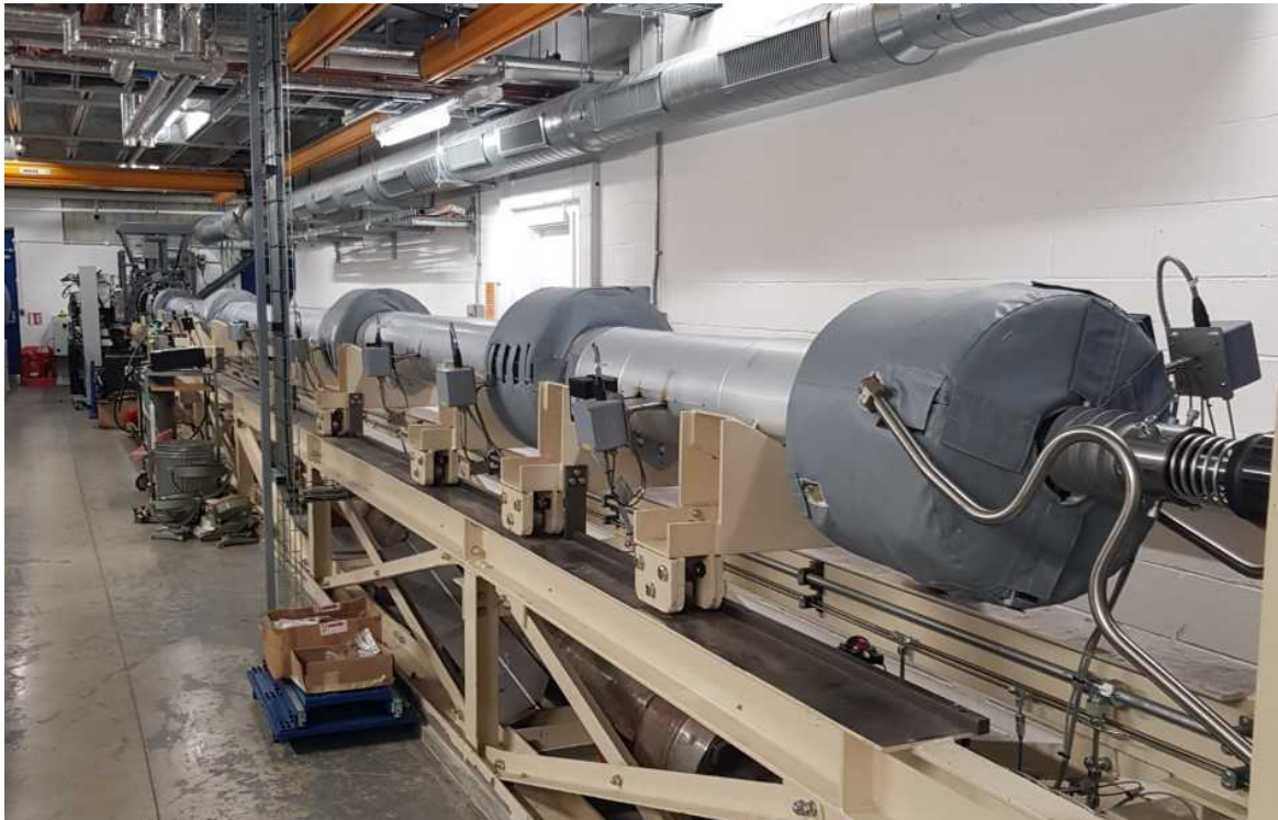
Fig. 3.9 Photo of the University of Oxford High Density Tunnel, test section can be seen at the far end of the facility
