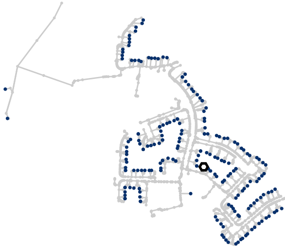
Figure 5.2: The Augmented EU LV (EULVa) network has 4 feeders connected to the same secondary substation; the EU LV network is to the Southeast of the substation.
