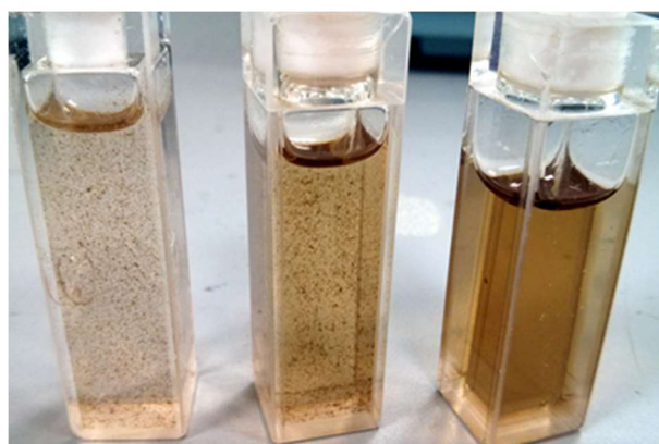
Figure 5.2-1 Photograph of 0.5mg/ml CZTS-toluene NC solutions, displayed left to right, synthesised with OLA/OA ligand ratios of 1:0, 11:1 and 5:1 respectively. Increasing the concentration of OA, relative to the OLA, had the effect of stabilising CZTS NCs in toluene, as is demonstrated by a reduction in the formation of solid aggregates and the deepening colour of the CZTS-toluene solution (from left to right).
