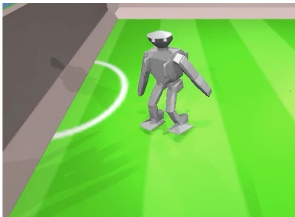
Figure 7.A.2: The OP 3 locomotion environment. The 20 DoF humanoid robot can walk around on a plane. The episode terminates early, if the OP 3 is about to fall over.
