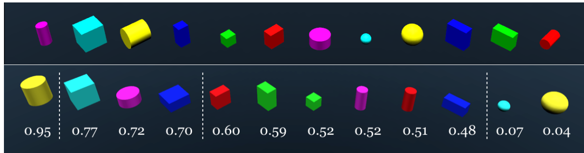
Figure 3.5: Top row: An unordered set of objects with random orientations. Bottom row: objects sorted from most stackable (left) to least stackable (right). Every object is oriented in the way which affords best stackability according to our network. The scores allow for division between different stability categories as visualised with white vertical lines.
