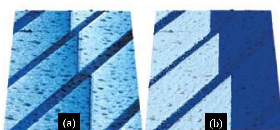
Figure 4.8: (a) PFM amplitude and (b) PFM phase overlaid on a AFM topograph showing 90^\circ and 180^\circ domain walls in single crystal \text{BaTiO}_3 (10 \mu\text{m} scan) (after Proksh and Kalinin, 2009 [156])
