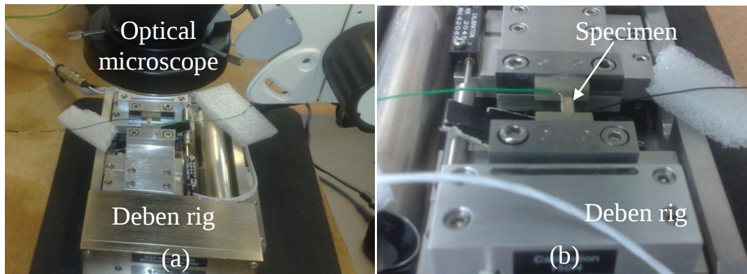
Figure 6.2: In-situ electromechanical testing using optical microscopy.
