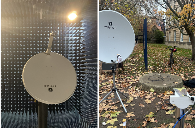
(a) Primary antenna under test in near-field range. (b) SIDEISH targeted by attacker antenna in urban environment.
