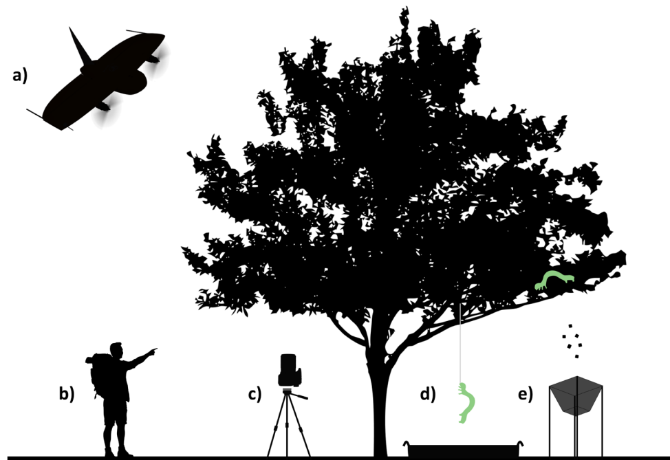
FIGURE 2 | Schematic of field methods performed on each tree: (a) multispectral drone imaging, (b) bud scoring observations, (c) hemispherical canopy photography, (d) caterpillar water traps, and (e) frass traps.
