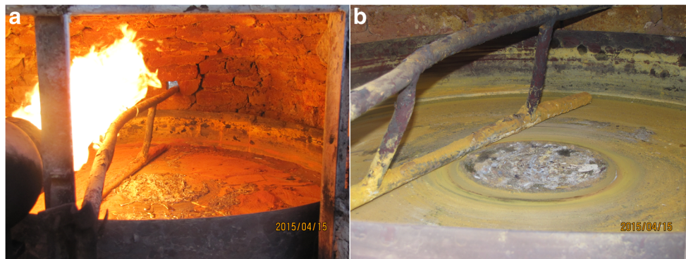
Fig. 6 The mixture of lead with tin heated for a 20 min showing the melt mixed with grey powder and b 80 min showing yellow calx powder
