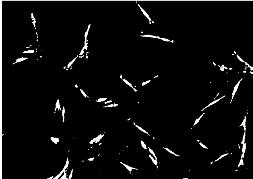
Figure 9-5: Thresholding the grayscale image into a two-tone image
