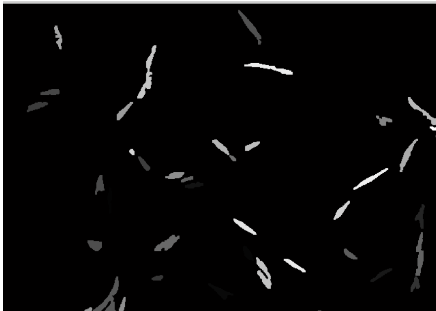
Figure 9-6: Elimination of objects smaller than 1200 pixels using morphological opening. In this image, each identified object is labelled with a different intensity of grey.
