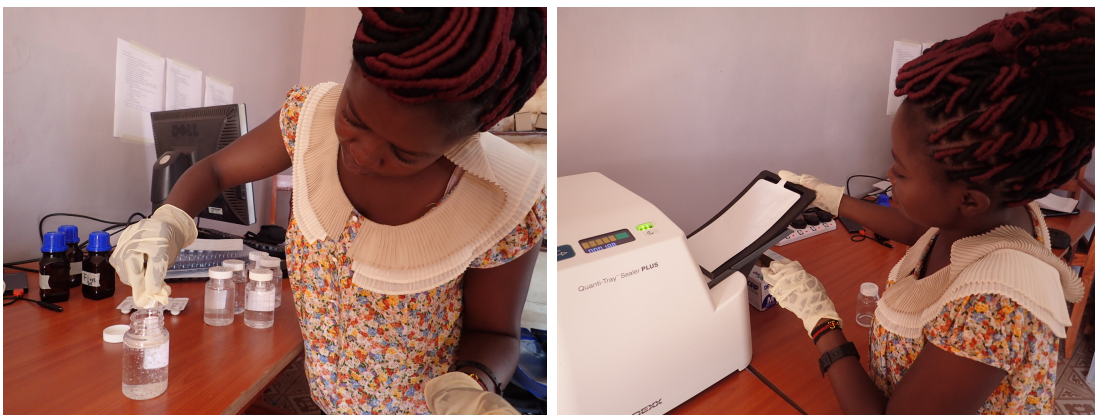
Adding Colilert-18 to a sample and feeding a quanti-tray through the sealer.
