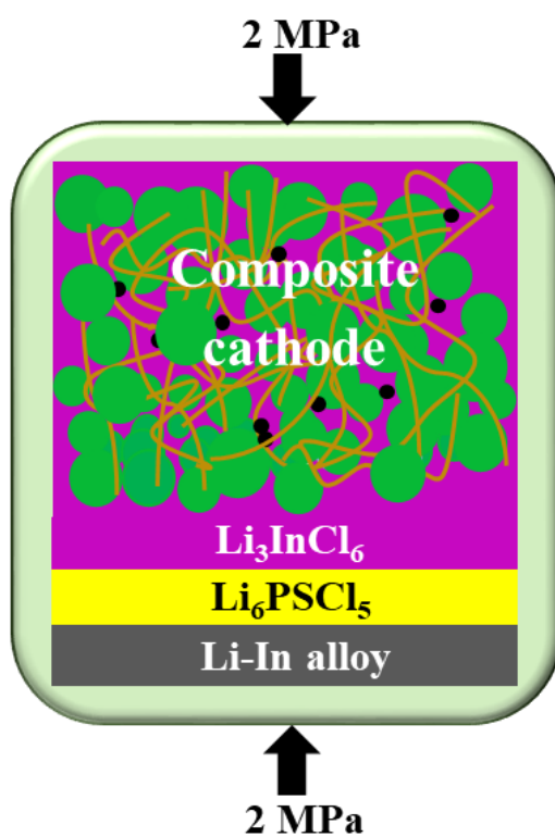
Figure S2. Schematic of the solid-state cell comprising a composite cathode, a layer of \text{Li}_3\text{InCl}_6 , a layer of \text{Li}_6\text{P}_5\text{Cl}_5 and a Li-In alloy.
