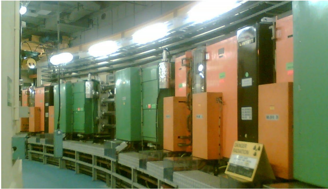
Figure 3: The PSB. Most of the beam-pipes are encased in magnets and RF cavities, but the four pipes can be seen towards the left of the photo.
