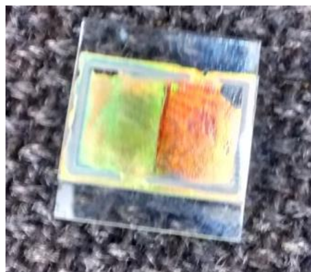
Figure 13 – A stretchable gel sample before delamination; it exhibits two regions with photonic band-gaps in different positions.
