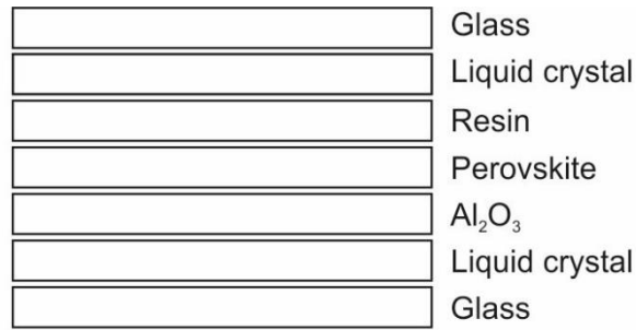
Figure 15 – A layered structure with perovskite sandwiched between two polymerised chiral nematic liquid crystal reflector layers.
