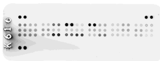
Figure S5. A LI-COR image of a membrane showing autofluorescent contamination from the ink in the serial number. The serial number must be removed prior to preparation.
